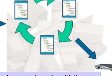
The receiver must sincronize with the beginning of a new transmission cycle of the carousel in order to download the file system that is contained in the stream
