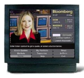
All the data and the application itself are broadcasted with the TV stream so the service is available to the users even when off-line (no TCP/IP links)
